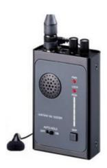
This is a professional portable audio bug detector is capable of detecting any conventional audio device transmitting from 30MHz – 900MHz. Detecting methods include a bar graph, audible verification and vibration making it useable in all environments. The Verifier is very easy to use and can be utilised in offices, homes and even vehicles.
